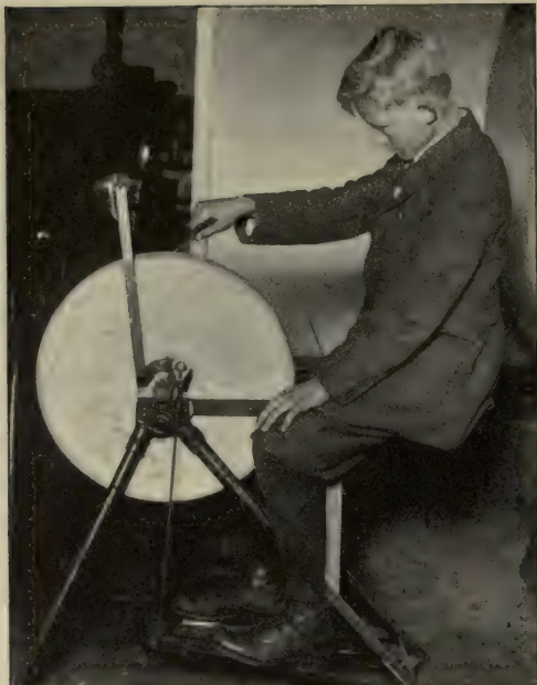
FIG. 25. The friction of the stone heats the nail and wears it away.
